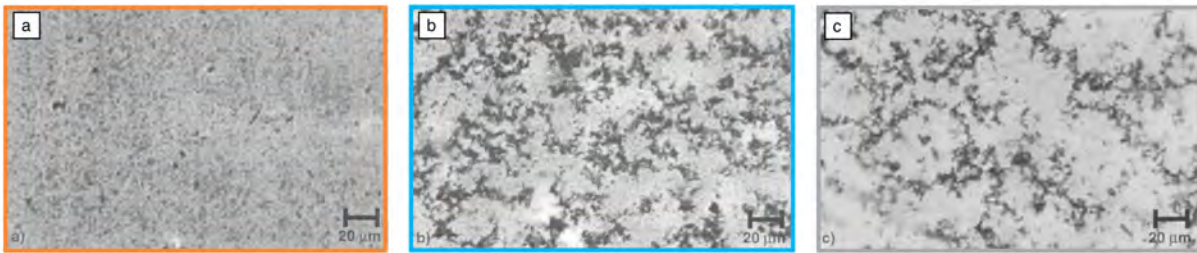
Figure 20. a) 0.6 vol.% CB-epoxy nanocomposite cured after mixing, b) 0.3 vol.% CB-epoxy nanocomposite cured after mixing with light shearing before curing, and c) 0.06 vol.% CB-epoxy nanocomposite with \text{CuCl}_2 [47].
