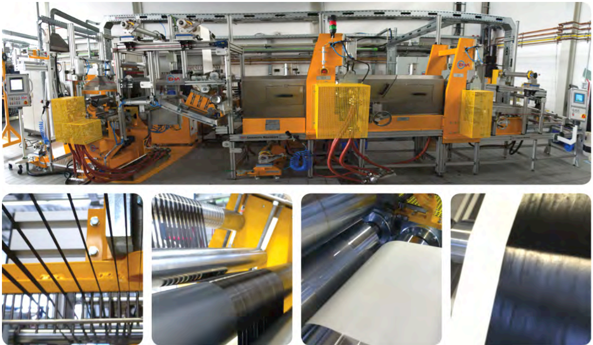
Figure 38. Laboratory-scale prepreg impregnation machine at the Department of Polymer Engineering. Below, left to right: roving organization, fiber pre-spreading, resin coating, and a final prepreg.
